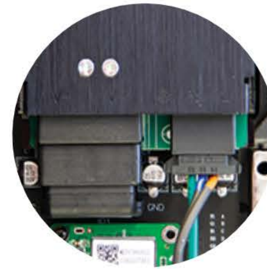
Power Supply Plug in place system
